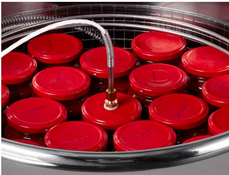
Temperature probe placed in one of the containers
